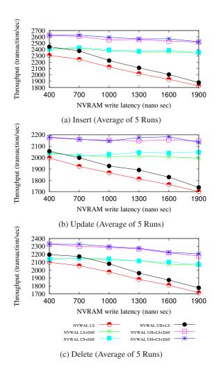
Figure 7: Transaction throughput with varying latency of NVRAM (Average of 5 runs on Tuna)
