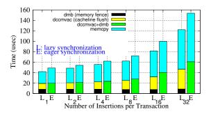
Figure 5: Quantifying the benefit of allowing processors to reorder memory writes
