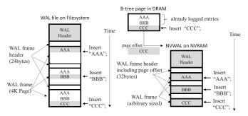
(a) Write-Ahead Logging in SQLite (b) Byte Addressable Differential Logging
