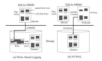
Figure 1: Write-Ahead Logging in NVRAM
